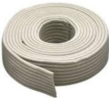
Rope caulk can be used to fill gaps primarily around windows, as a temporary measure to stop air flow. Rope caulk sticks in place and can be removed easily. First, clean the area where you will use the rope caulk, to prevent any dirt or grime from making the rope caulk less sticky and, as a result, less able to seal properly. Next, tear off the amount of rope caulk you need to fill the space. Finally, firmly press the strand of rope caulk into the gap or crack you wish to fill.
